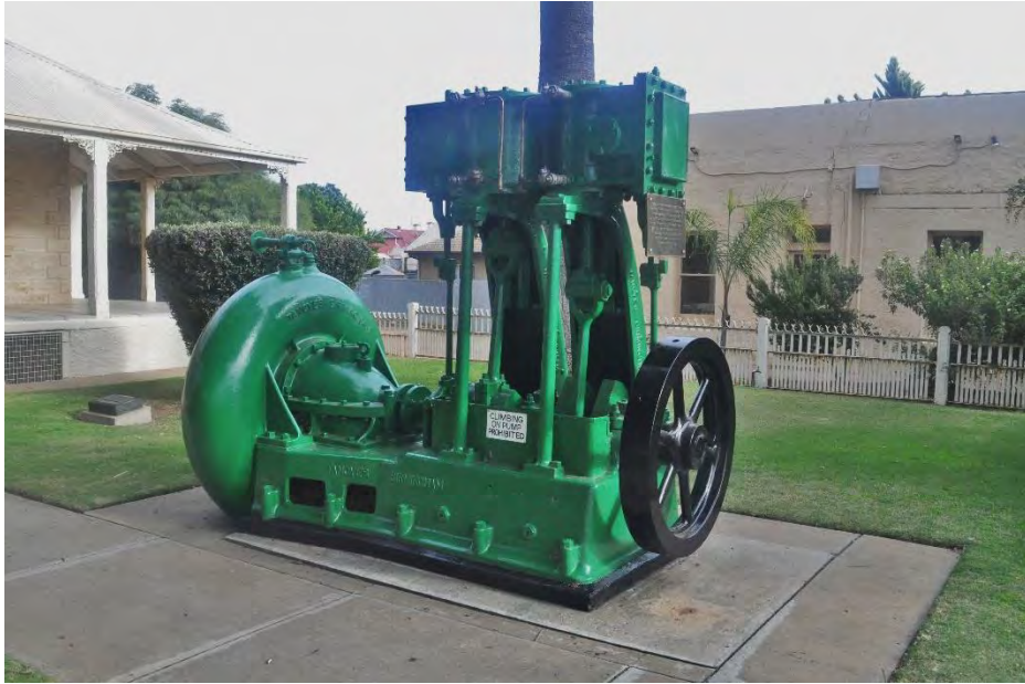
Tangye, Birmingham steam pumping engine at the Renmark Irrigation Trust Office. Image: Owen Peake.
